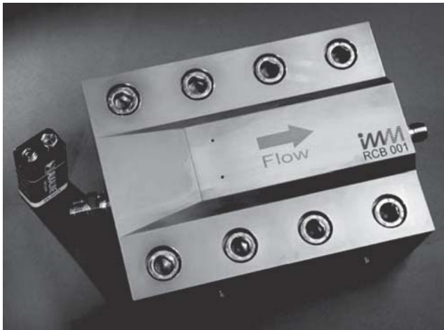
Fig. 3 Stacklike testing reactor for catalytic combustion of methanol
